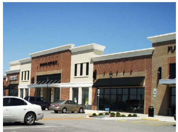
The parapet on this building modulates; cornices correctly return at least 8 feet at exterior corners.
